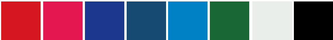
Traffic Red RAL3020 Strawberry Red RAL3018 Ultramarine Blue RAL5002 Violet Blue RAL5000 Sky Blue RAL5015 Leaf Green RAL6002 Signal White RAL9003 Jet Black RAL9005
